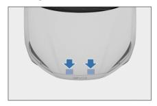
4. After closing the hood, check whether the latch is securely locked.
