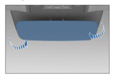
· Anti-glare mode - adjust the control lever in position, where the interference from headlights behind can be effectively reduced at night. Remember that rear view image clarity decreases when glare is reduced.
