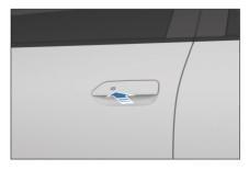
· When the vehicle cannot be waked up and unlocked by the driver door microswitch, use the mechanical key to open the door. Then, a 12V power
