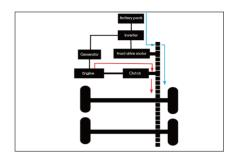
In HEV mode, the engine drives the vehicle and simultaneously drives the motor to generate electricity for energy recycling.
