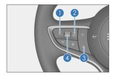
Activate the ACC function by pressing the key ③, and the system will actively set the current vehicle speed as the target cruising speed (if the current vehicle speed is less than 30 km/h, the target cruising speed will be set as 30 km/h); activate the ACC function by pressing the up key 4, and the target cruise speed will be set as the vehicle speed set before the function was exited last time.
