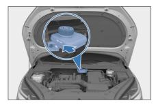
If the fluid level is at or below the lowest limit (MIN) mark, it is necessary to check the brake system for leakage and wear of brake friction plates.
