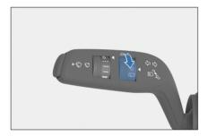
• To operate the wiper in the spot mode, press the button at the end of the operating lever to the first gear position, and the wiper will hang water at a low speed until the button is released.
