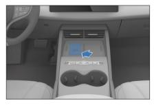
· Wireless phone charging uses a coil to transmit electrical energy to a phone battery through electromagnetic wave induction so that the phone can be charged without a cable connection.
