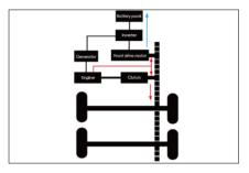
• In HEV mode, the engine drives the vehicle and the drive motor rests.
