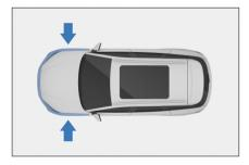
An impact to a vehicle door (shaded part in the figure) in an accident is not adequate to cause the airbag to deploy.
