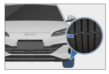
Replace the tire if the tread is worn to the extent that the wear mark is exposed, in which case the tire performance is greatly lost.
