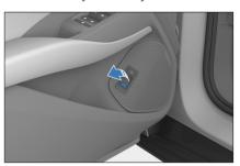
With the vehicle powered on and the trunk open, pull this switch for more than one second to automatically close the trunk. Release the switch to freeze the closing motion.
