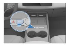
Pressing the accelerator pedal, shifting into Park, or engaging the EPB can make AVH exit to the standby status. The vehicle exits AVH mode even if the AVH standby conditions are not met.
