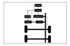
In HEV mode, the engine and the high-voltage battery simultaneously supply power to the drive motor.
