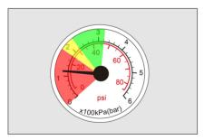
If the tire pressure reaches 180~320 kPa (green and yellow areas shown in the illustration), remove the kit as soon as possible and drive at a speed below 80 km/h within one minute, with the furthest driving distance not exceeding 10 km, so that the tire sealant is evenly distributed within the tire.
