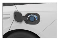
• If the fuel tank cap is idling and cannot be opened, contact a DENZA authorized dealer or service provider. Emergency opening of fuel filler cap: Lever the blanking cap off, which is in the center of the fuel tank cap handle. Insert a slender guide rod (such as a gel pen refill) into the small hole till the end and keep, and rotate the handle counterclockwise to take the fuel tank cap off.
