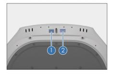
The side airbag warning labels are pasted on the lower part of left and right B pillars.
