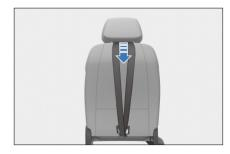
· When the child restraint is installed on a front passenger seat with a top tether, pass it through the gap in the headrest compartment.
