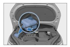
Motor controller coolant type\*
