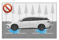
· Drive carefully as driving through deep water may wet the brakes. After driving through the flooded area, press the brake pedal several times continuously and gently to evaporate the water on the brake disc, so as to restore normal braking performance as soon as possible.
